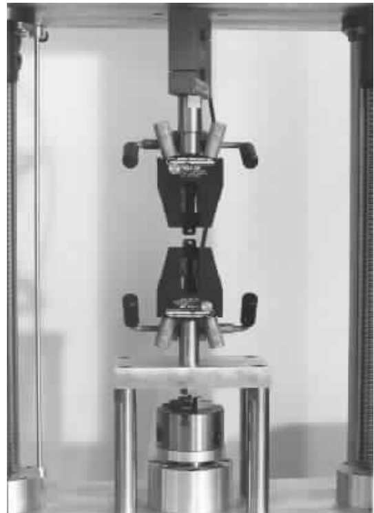
Figure 3 Setup Showing Wedge Type Tensile Testing Grips with Lower Axial Loading Platform Installed
