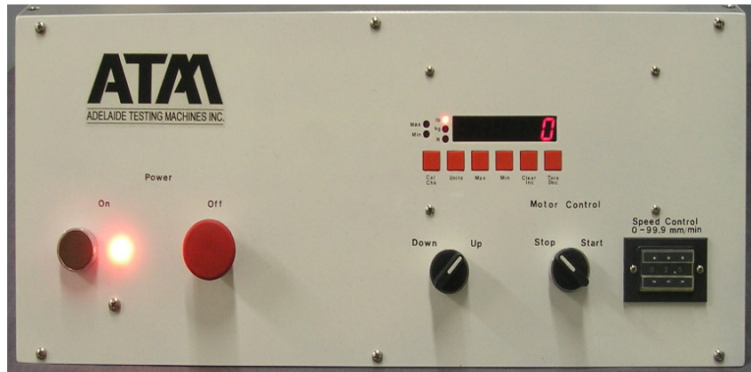
Figure 2 Front Panel Showing AC Power and Motor Control Switches
