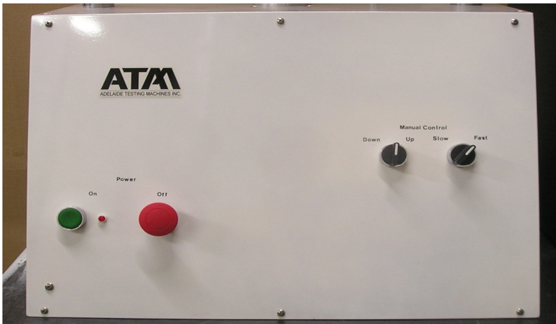
Figure 3 Control Switches on Front Panel
