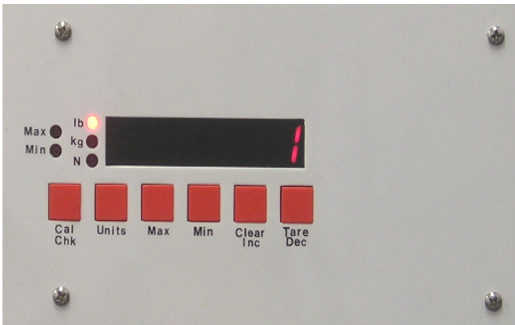
Figure 4 View of Microprocessor Display for Load Indication
